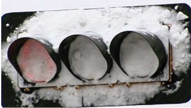
Figure 1. A snow-covered LED traffic light, such as the one included in the Traffic Light Problem (colour online).
