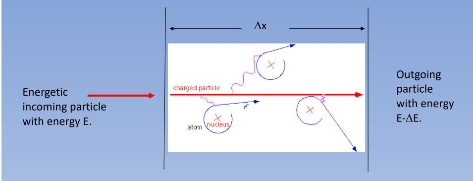
In detectors, the ions are counted somehow. The ions usually don't last long because the electrons find an ion with which to recombine. The bonding process liberates photons (light) that can be detected. By detecting the light of recombination, we can infer the energy loss,  $\Delta E$ , of the incident particle.
