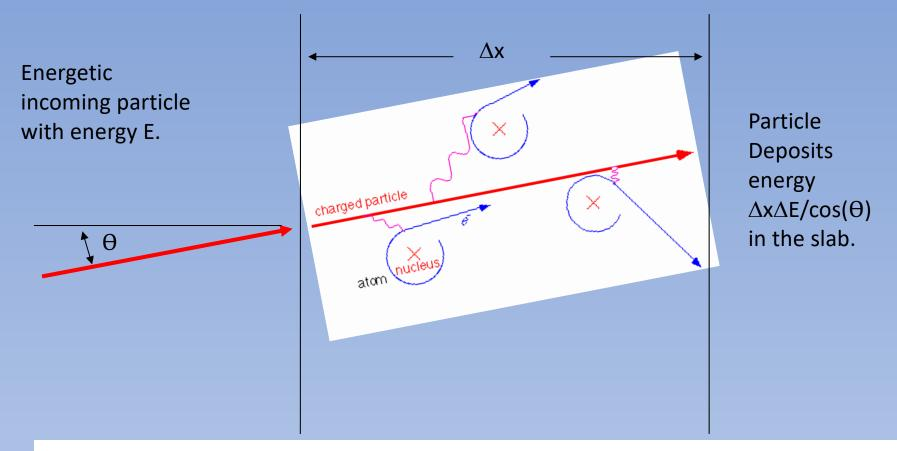
Our detectors were slabs of plastic,  $\Delta x$  about 1 cm thick, doped with what were called scintillating chemicals that grabbed the energies of recombination and turned it into visible light.
