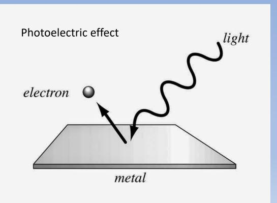
If the layer of metal is thin, the electron can leave through either surface.
