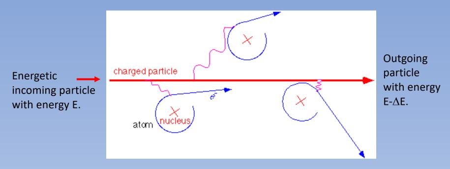
Xs represent atomic nuclei and the blue represent orbital electrons. After the passage of the energetic particle, the medium is ionized and the incoming particle has a little less energy.
