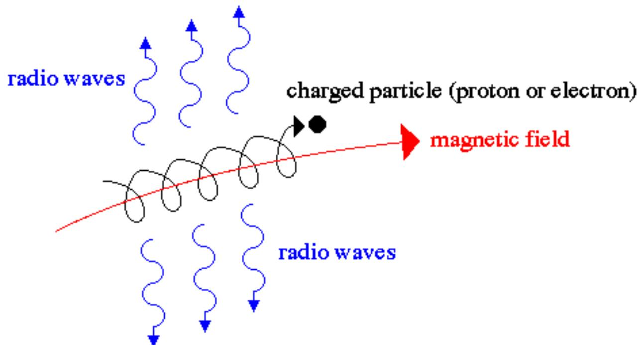
synchrotron radiation occurs when a charged particle encounters a strong magnetic field – the particle is accelerated along a spiral path following the magnetic field and emitting radio waves in the process – the result is a distinct radio signature that reveals the strength of the magnetic field
